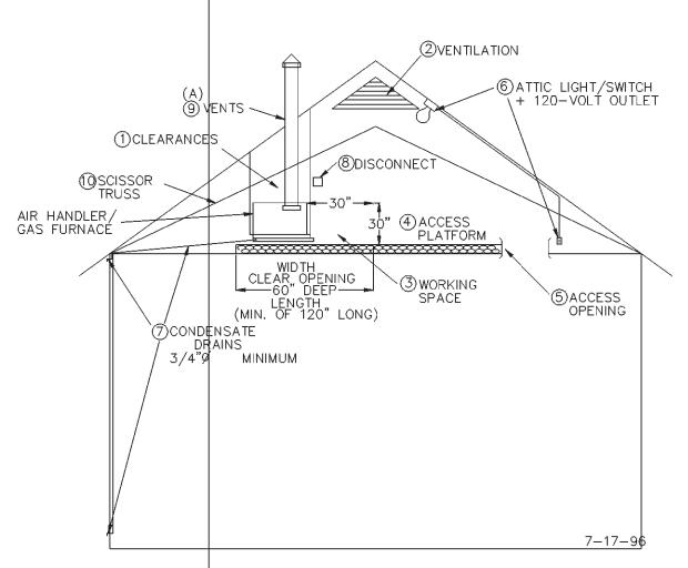
REQUIREMENTS FOR ATTIC AIR HANDLER OR GAS FURNACE 1. CLEARANCES FROM COMBUSTABLE MATERIALS FOR GAS FIRED FURNACES MUST BE AS SPECIFIED IN THE MANUFACTURER'S INSTALLATION INSTRUCTIONS AND APPLICABLE LOCAL BUILDING CODES. (A)
