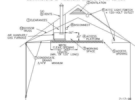
REQUIREMENTS FOR ATTIC AIR HANDLER OR GAS FURNACE 1. CLEARANCES FROM COMBUSTABLE MATERIALS FOR GAS FIRED FURNACES MUST BE AS SPECIFIED IN THE MANUFACTURER'S INSTALLATION INSTRUCTIONS AND APPLICABLE LOCAL BUILDING CODES. (A)
